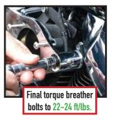
4. On the inside of the filter cage, see "S" for Softail & "T" for Touring models. Align this bolt hole to the top left bolt hole of backing plate, this will clock the cage and logo properly. Install velocity stack, gaskets and bolts.
