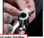
Lube and install inner and outer breather 0-rings, use with 0-ring lube.
