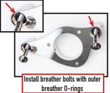
3. If throttle body bracket is removed, use included spacers. If bracket is present (preferred), no need to use the included spacers. Install breather bolts with red loctite on threads & 0-ring lube on underhead flanges. Insert velocity stack bolts to help center backing plate. Alternatley tighten and torque breather bolts. Final torque to 22–24 ft/lbs.
